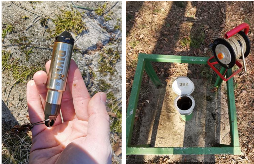
Figure 32. Groundwater level measuring devices in Latvia (on the left - automatic water level datalogger; on the right - manual water level meter)
