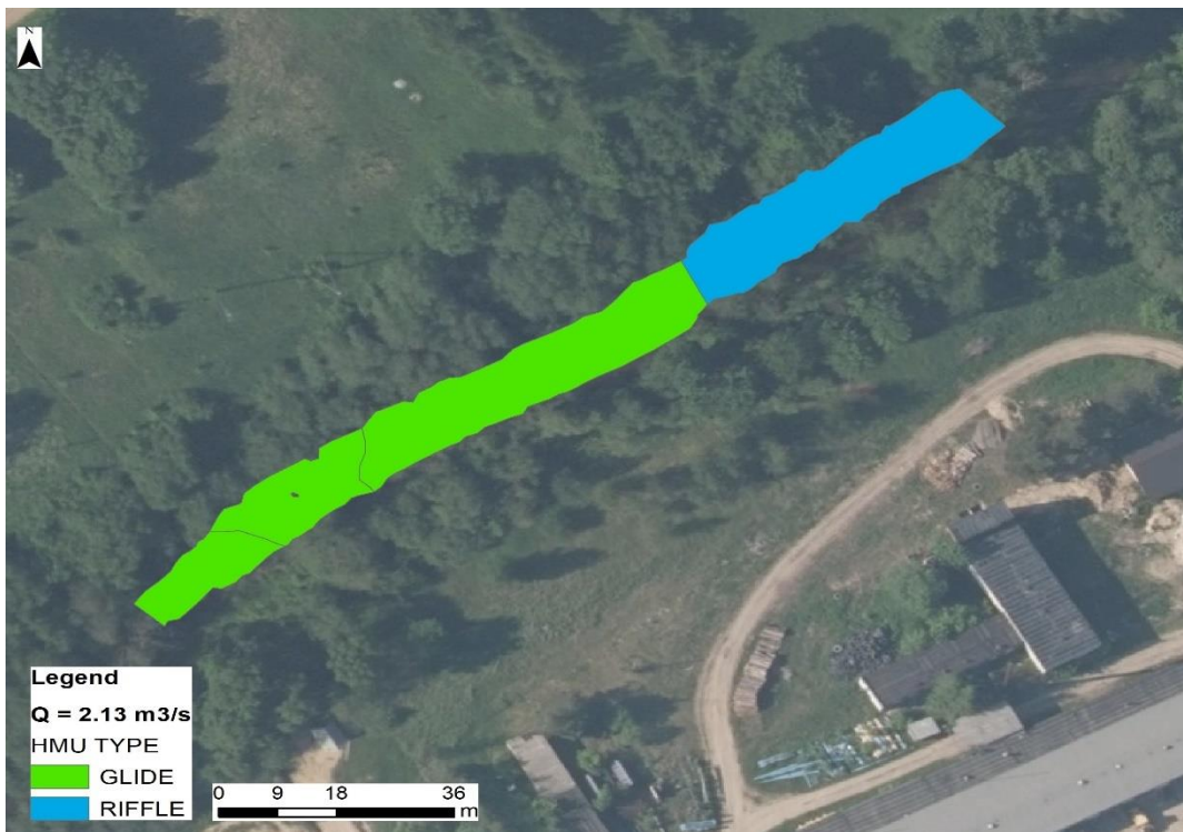
Figure 8. Hydromorphic unit map of the Ciecere 2 (below Saldus city) River below Dzirnavnieki HPP ( Q = 2.13 \text{ m}^3/\text{s} )
