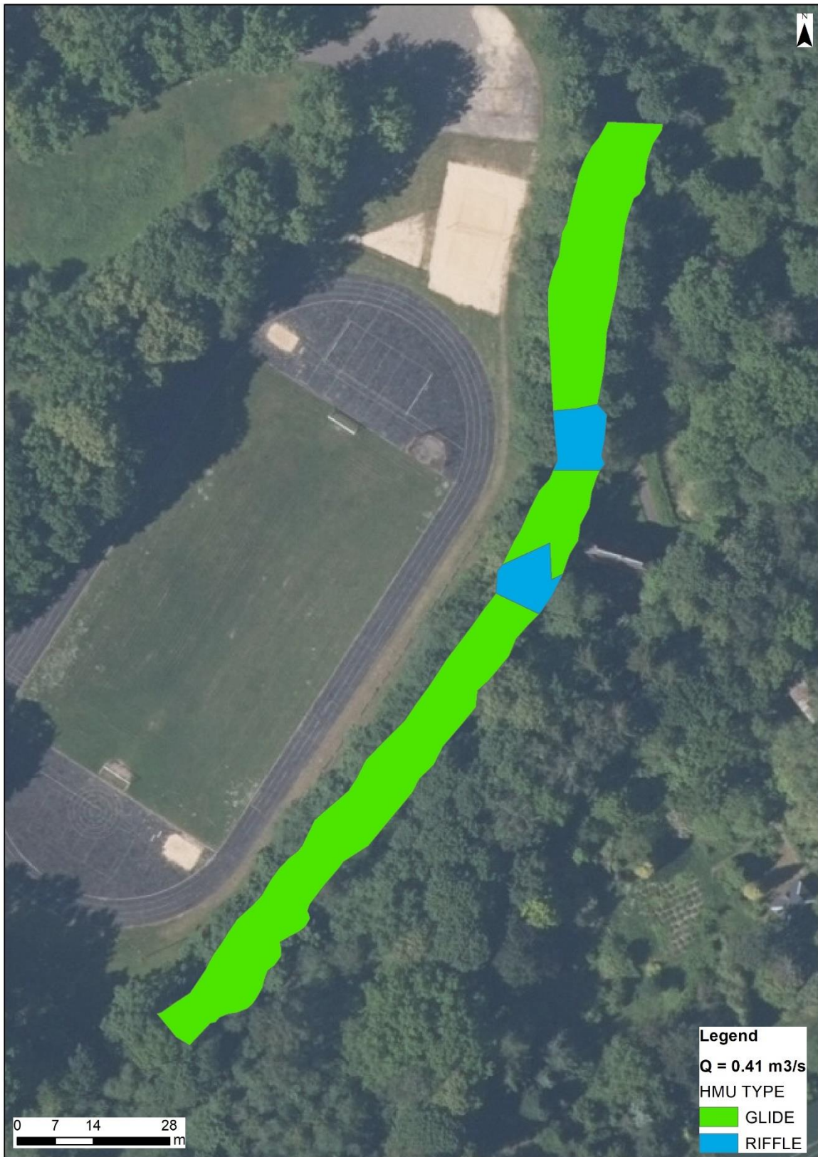
Figure 19. Hydromorphic unit map of the Losis 2 River below Grantini HPP ( Q = 0.41 \text{ m}^3/\text{s} )
