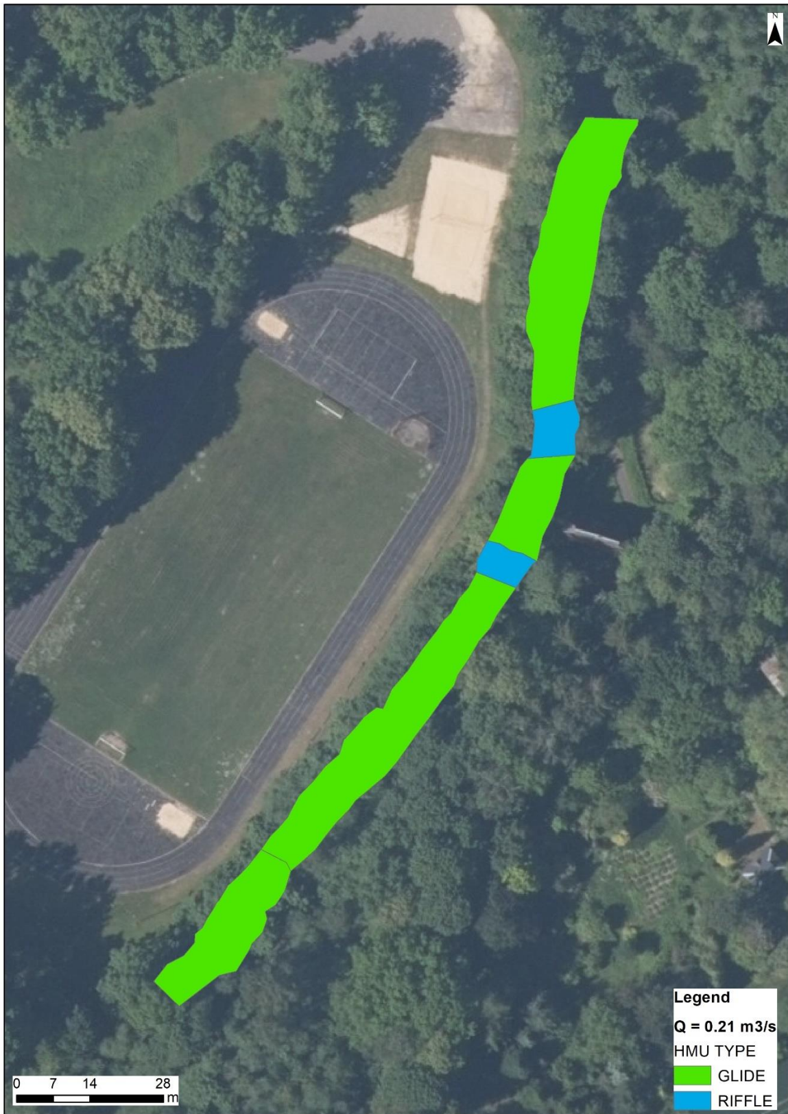
Figure 18. Hydromorphic unit map of the Losis 2 River below Grantini HPP ( Q = 0.21 \text{ m}^3/\text{s} )
