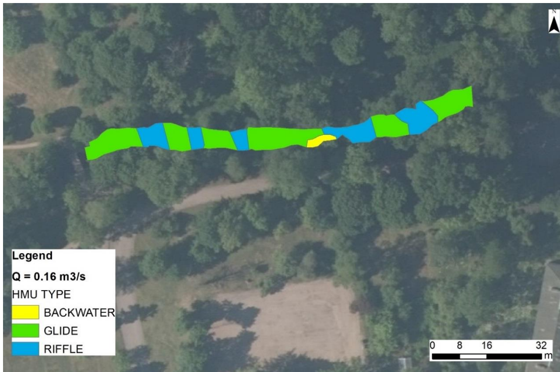
Figure 1. Hydromorphic unit map of the Ciecere 1 (at Kalnsetas parks) River below Ciecere HPP ( Q = 0.16 \text{ m}^3/\text{s} )
