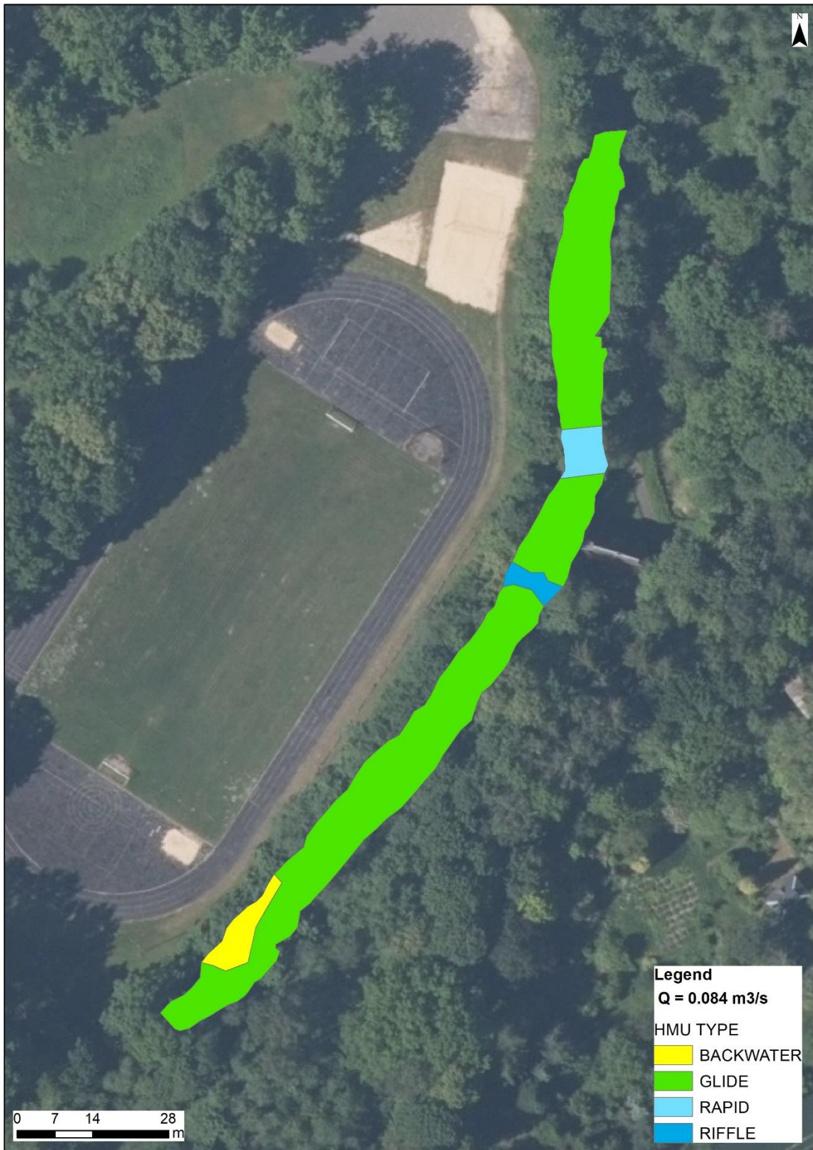
Figure 17. Hydromorphic unit map of the Losis 2 River below Grantini HPP (Q = 0.084 m 3 /s)
