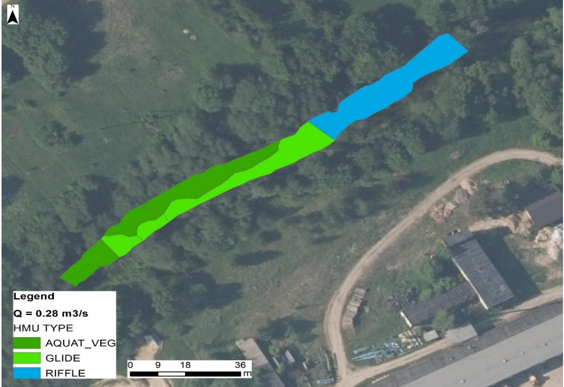
Figure 6.. Hydromorphic unit map of the Ciecere 2 (below Saldus city) River below Dzirnavnieki HPP ( Q = 0.28 \text{ m}^3/\text{s} )
