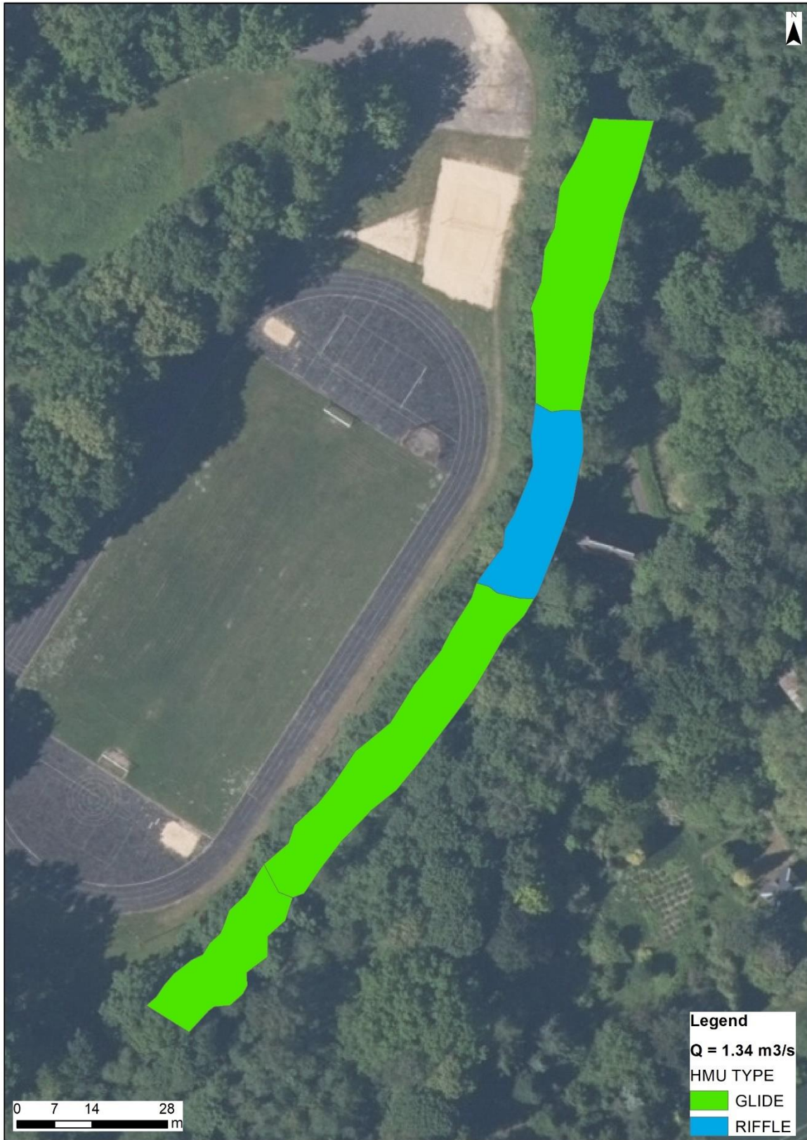
Figure 20. Hydromorphic unit map of the Losis 2 River below Grantini HPP ( Q = 1.34 \text{ m}^3/\text{s} )
