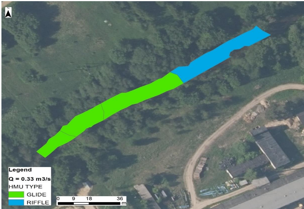
Figure 7. Hydromorphic unit map of the Ciecere 2 (below Saldus city) River below Dzirnavnieki HPP ( Q = 0.33 \text{ m}^3/\text{s} )
