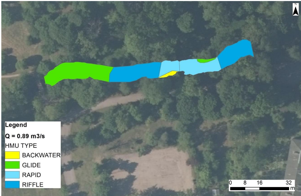
Figure 3. Hydromorphic unit map of the Ciecere 1 (at Kalnsetas parks) River below Ciecere HPP (Q = 0.89 m 3 /s)
