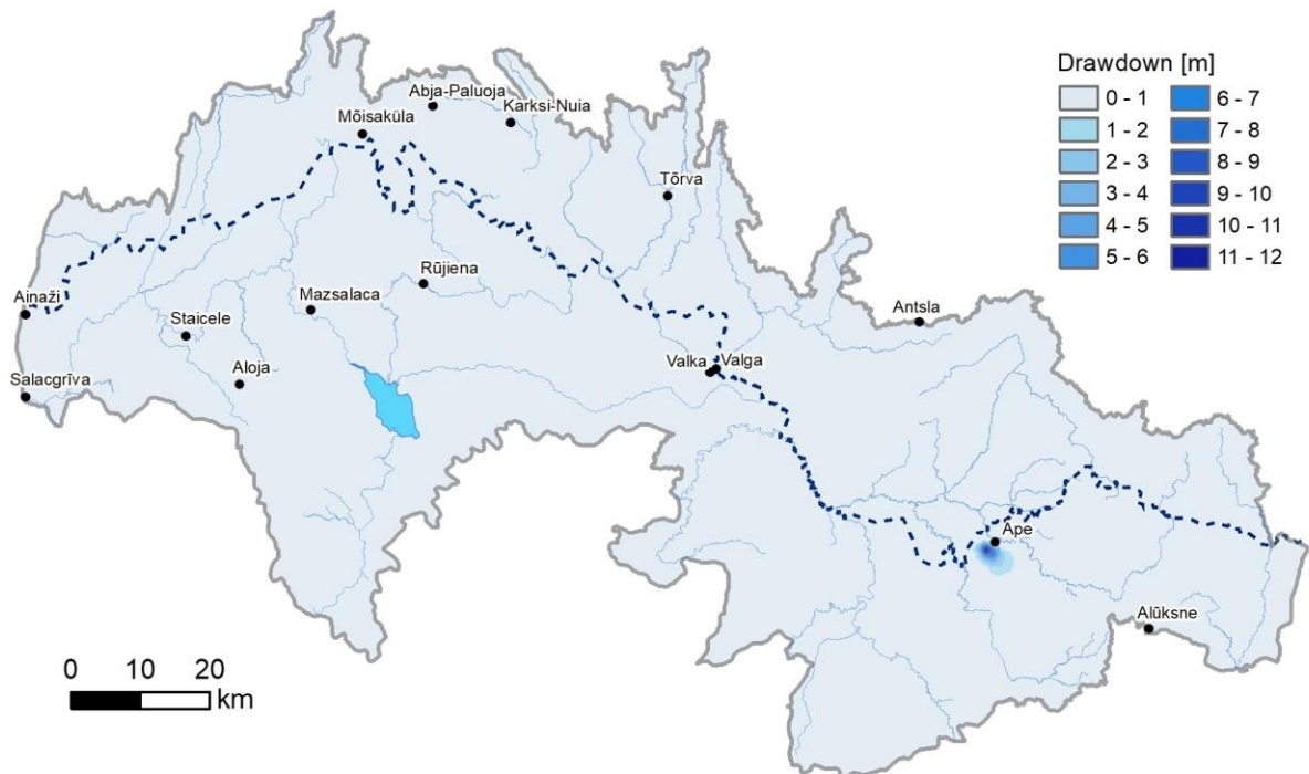
Figure 62. Simulated groundwater drawdown with current exploitation rate from 2012–2021 (represents all three aquifer systems)
