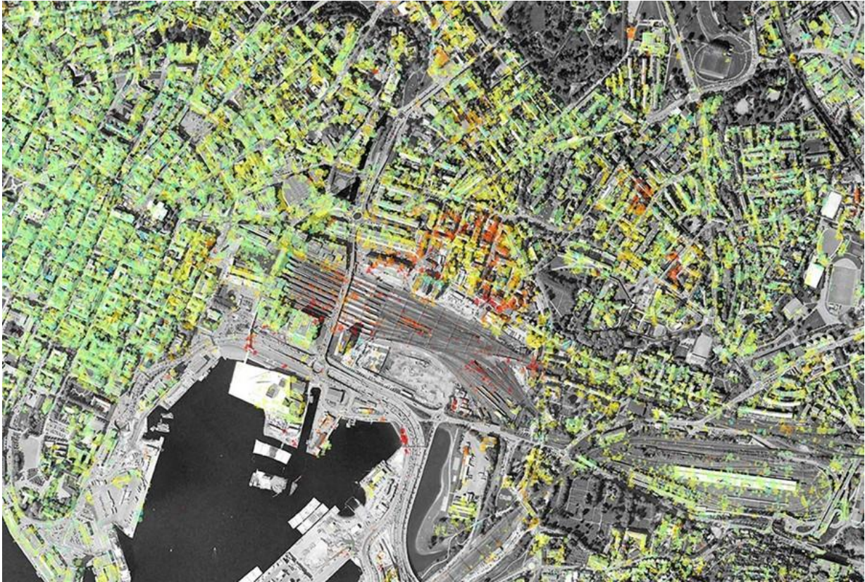
Figure 6. Oslo city centre, analysis of InSAR images between 2009 and today reveals more than one centimetre per year of subsidence in the Bjørvika area
